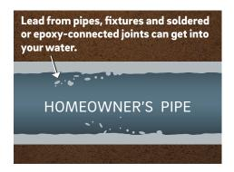
As water stands in your home's plumbing, lead from soldered joints, lead epoxy and old lead pipes can get into your water. Other debris can build up on the aerator, too. It's important to clean faucet aerators and screens to remove any debris from them.
